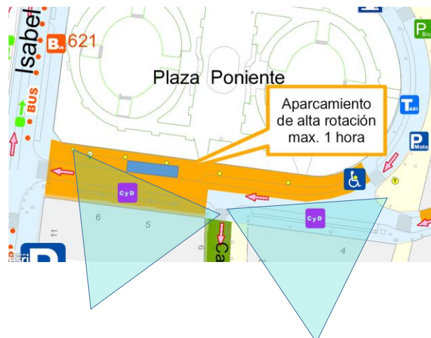
FIGURE 13. LOCATION OF THE L/U ZONES AND THE VIDEO CAMERAS INSIDE THE OPERATIONAL AREA
