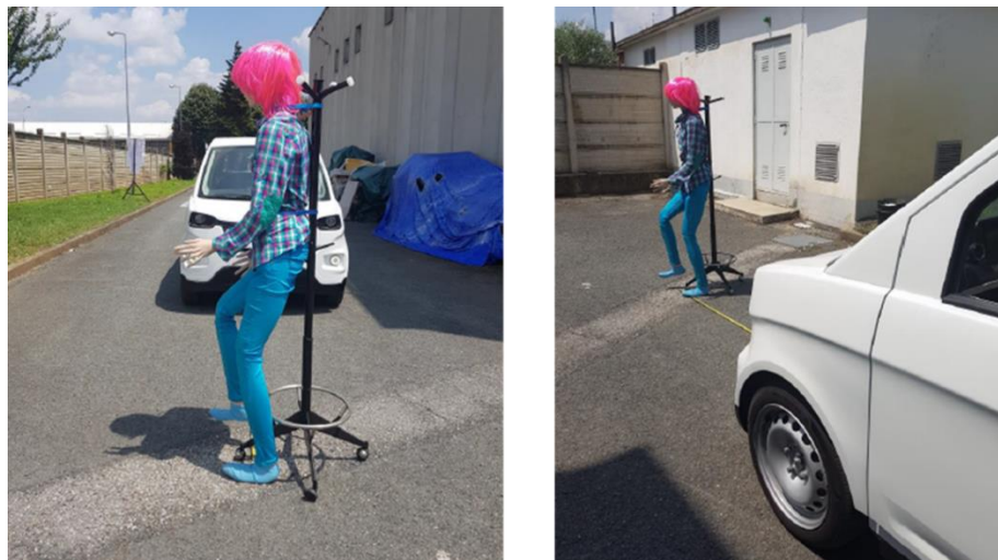
FIGURE 29. VALIDATION TESTS CARRIED OUT DURING THE DEVELOPMENT OF THE PEDESTRIAN DETECTION SYSTEM
